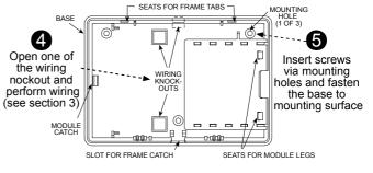
Securing the Base to a Wall or Host System Cabinet
