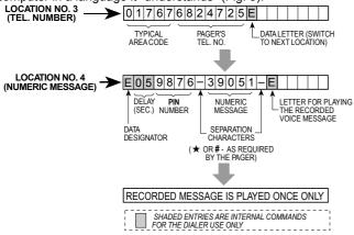
Figure 5. Typical Data Arrangement in Memory
